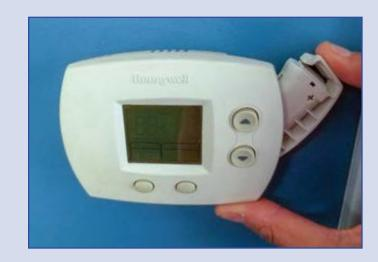
Most digital thermostats are programmed to display a low battery warning one or two months before the batteries go dead. This gives you some time to purchase new batteries, but don't wait too long! When your thermostat loses power it can cause your heating or cooling system to shut off.
